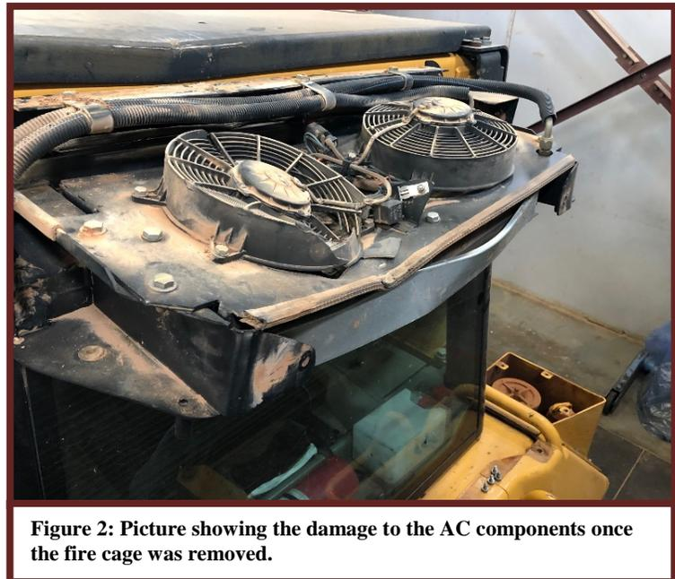
**Figure 2: Picture showing the damage to the AC components once the fire cage was removed.**
