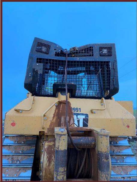
**Figure 1: Winch line ran over the dozer cab to attempt the lift the disabled blade.**
