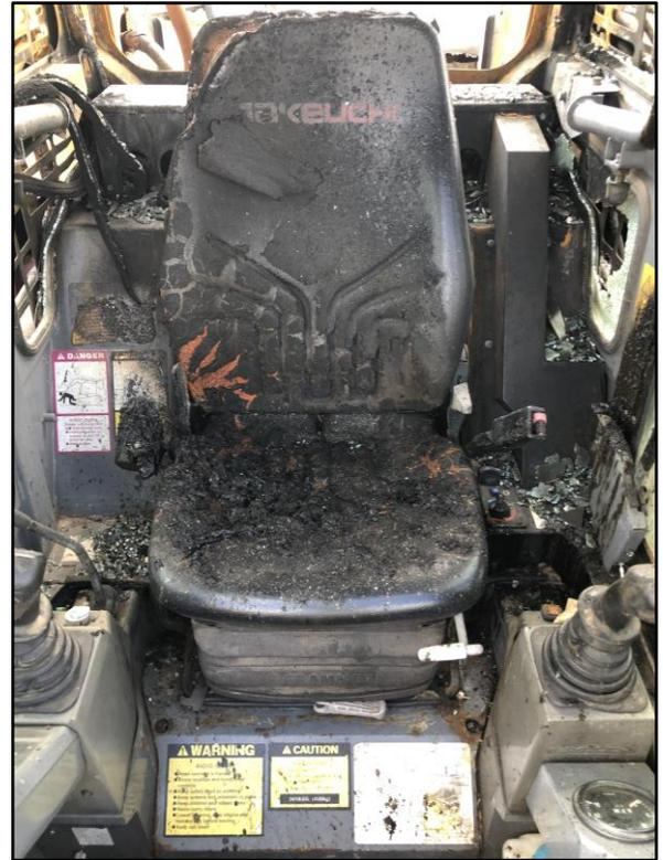
Picture 3: Operator's seat in Takeuchi after incident
