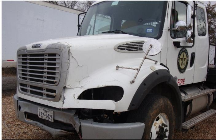
*The damaged transport. A limb penetrated into the engine compartment causing damage*
