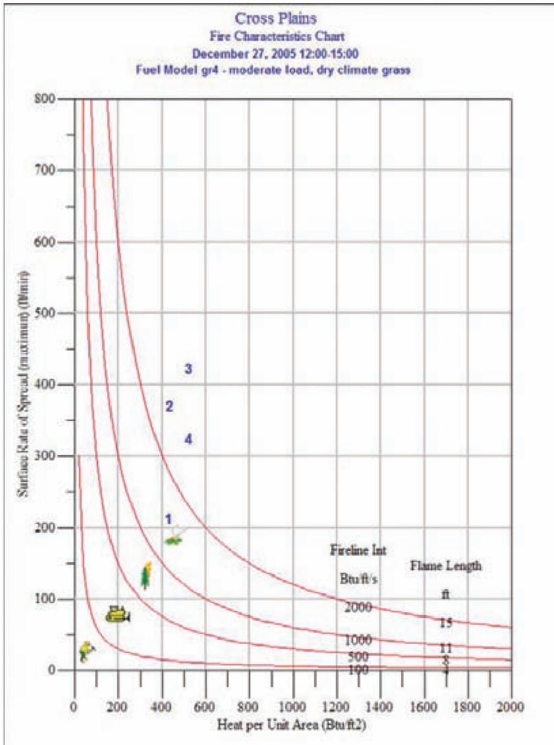
Figure 10 – Fire characteristics chart created in Behave Plus using the gr4 fuel model and weather data from the Hamby RAWS.
