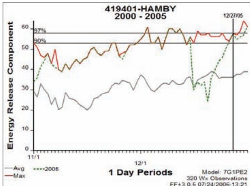
Figure 7 – ERC values calculated by Fire Family Plus using data from the Hamby RAWS, Nov. 1 - Dec. 31, 2005.
