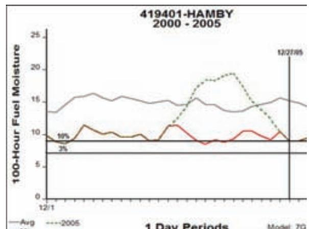
Figure 5 – 100-hour time lag fuel moistures calculated by Fire Family Plus using data from the Hamby RAWS Dec. 1 - Dec. 31, 2005.
