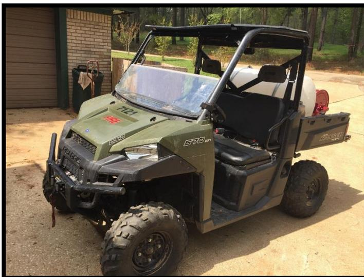
*The UTV after return to the local office. Note the bow in the roof from the roll over.*
